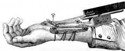
Fig. 109. Sphygmographe direct.
